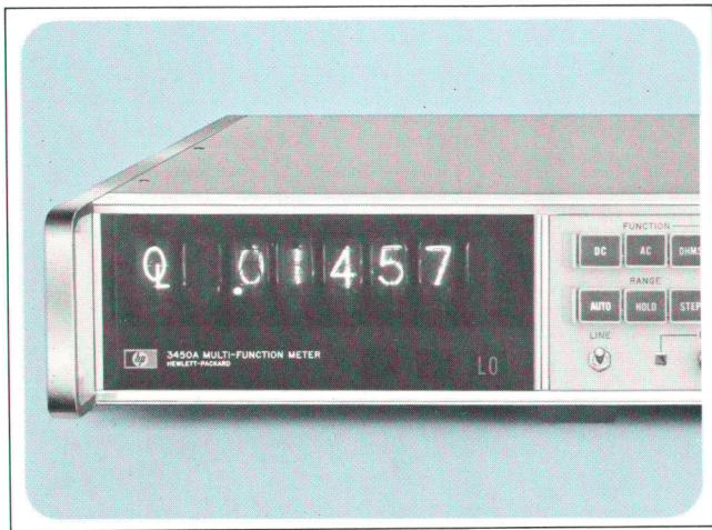
Fig. 11. Indication shows ratio underload on the HP Model 3450A when reference voltage drops below a usable level.
